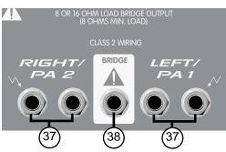
**CAUTION:** When using the bridge output no other speakers should be connected to the adjacent parallel speaker outputs. In addition, the minimum load for the XR 684 in bridge mode is 8 ohms. Do not allow the total impedance to drop below 8 ohms or serious damage to the amplifier may occur.
